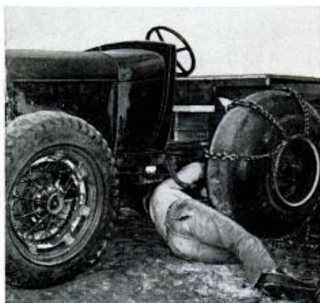
Chains help traction and are widely used on swamp buggies. Putting them on airplane tires is easy task
